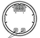
USED FOR DEVICE CONFIGURATION DO NOT CONNECT WHEN INSTALLING GAGE
