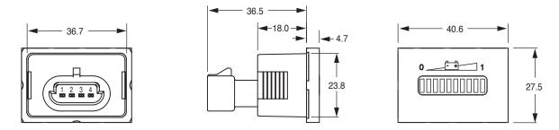
NOTE: Equivalent to Delphi-Packard connector P/N 15336035 4-pin.
