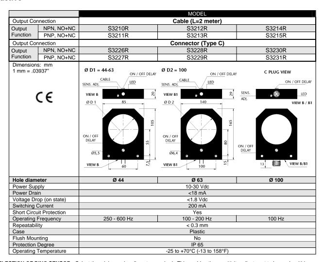
**SELECTION OF RING SENSOR:** Select the minimum ring diameter required. This enables the sensitivity adjustment to be made within normal parameters ensuring proper functioning of the unit.
